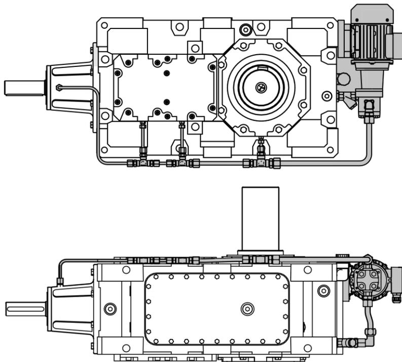
Motor pump for bearing lubrication supplied already mounted on the gear reducer (example for mounting position V6).
